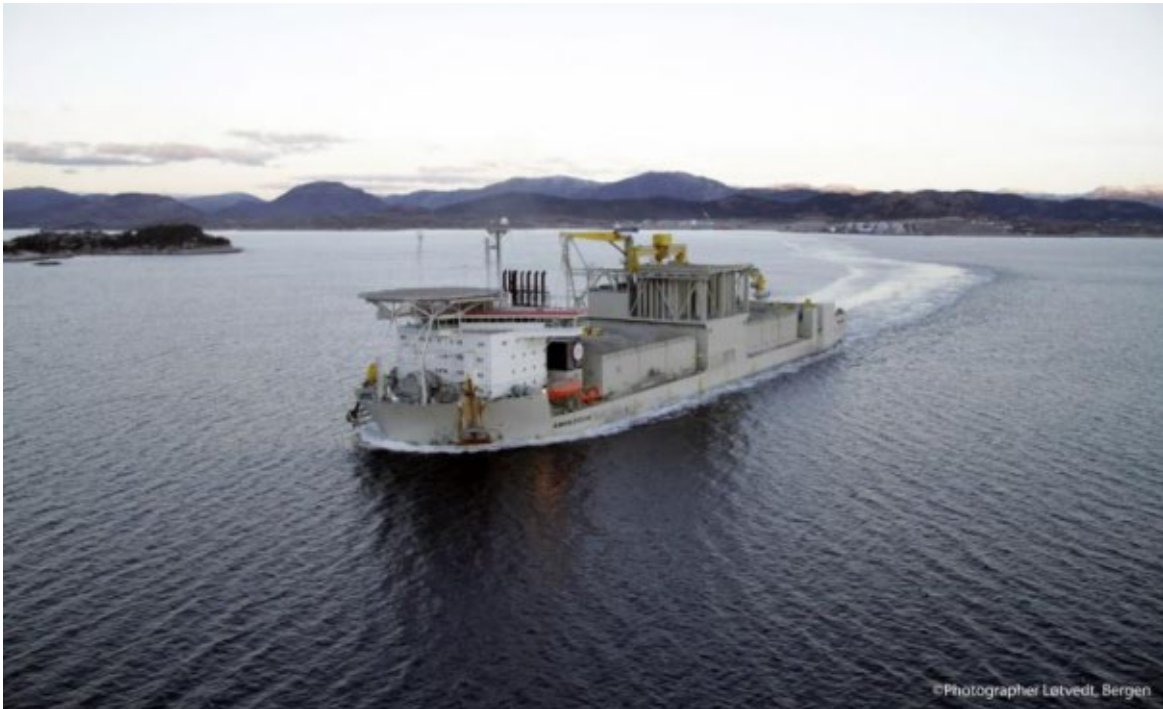
Plate 5.9 Indicative scour protection deployment vessel (source: Jan De Nul Group, 2023)
